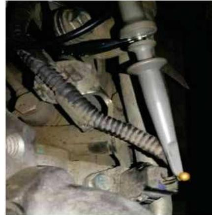
Fig. 5. Conector del sensor CKP.
